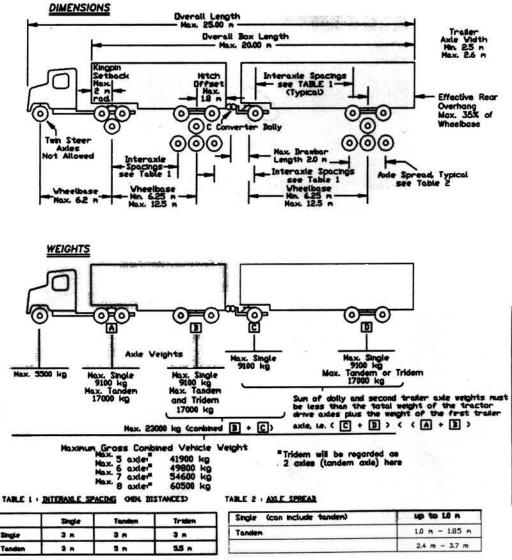
100 kg/cm the width applicable to all thres. Nax, 3000 kg/thre applicable to all axies except the steering axie which is limited to 5500 kg.
